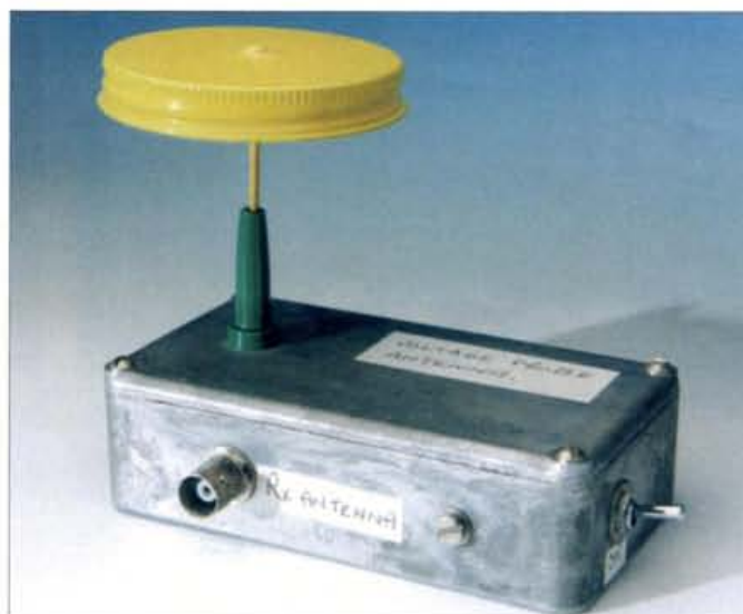
Fig. 1: Peter Buchan's Voltage Probe Antenna (v.p.a.) can outperform a wire antenna at low frequencies, see text for more details.
