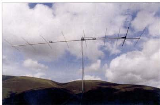
Fig. 1: The Tonna F9FT 9-element portable antenna which Phil uses for 144MHz
