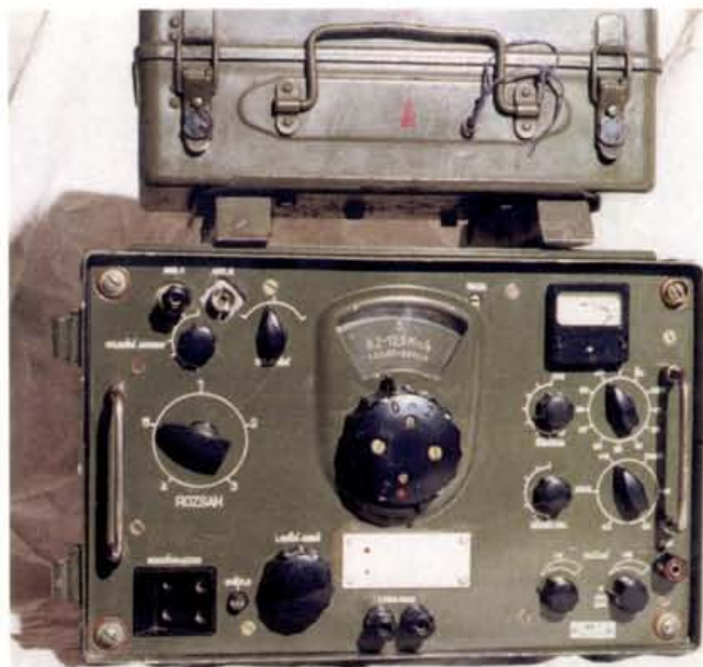
Fig. 2: The R4-1 receiver, main tuning lower left, with headphone sockets bottom left and S-meter/voltmeter top right. (The p.s.u. plugs in at the rear).
