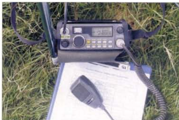
Fig. 2: Phil M0AYB uses a Yaesu FT-290 MkII 2.5W portable transceiver for his portable contesting.
