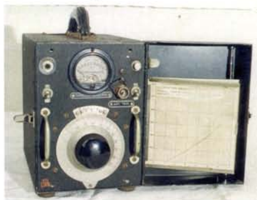
Fig. 4: The BC-906D Wavemeter with calibration chart housed in the lid. A small extendible whip antenna plugged into a socket on top of the meter's case.
