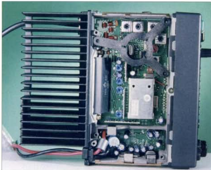
Fig. 2: Top view of the inside of the ADI AR-147 transceiver. The extensive (and efficient) heat-sinking is clearly shown, along with the innovative 'three legged' loudspeaker mounting assembly which considerably reduces case vibration at higher audio output levels (see text).
