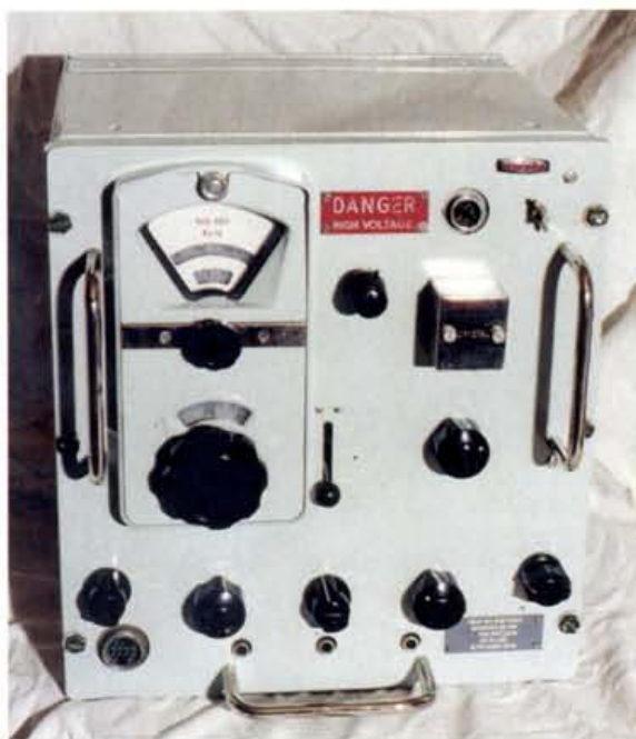
Fig. 1: The Murphy h.f. receiver. Because the control knob lettering is white, it doesn't show up too well in the photograph against the light blue paint work.
