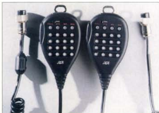
Fig. 1: Close-up photographs of the ADR microphones, clearly illustrating the complex functions provided (see text for comments on repeater working). The newer AR-147 microphone (left) is provided with a ferrite sleeve.
